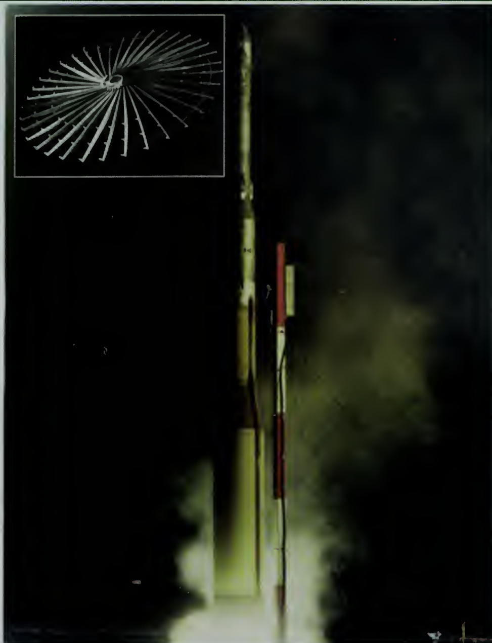
Fig. 3-10. Noted for its distinctive web (insert) designed to capture an RV, the Homing Overlay Experiment achieved the first kinetic energy intercept colliding with its target at a speed of 20,000 mph.
